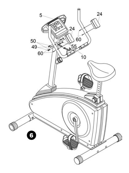
**6.** Attach the pulse wires in the handlebar (10) to the wires from the console (5). Connect the handlebar (10) to the console tube with the locknuts (49), flat washers (50) and screws (55) provided. Make sure not to "pinch" any of the pulse wires when connecting the handlebar to the console tube. Attach the elbow pads (24) to the handlebar (10) with screws (60).
